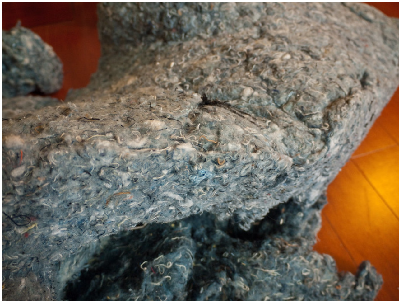
Figure 5.3.2 – Insulation material made from recycled cotton jeans
